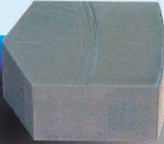
Micro- contour-artefact, calibrated by PTB
