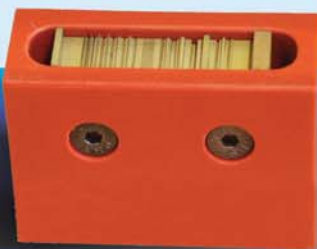
PTB calibrated micro artefact with steep flanks, height steps and cylindrical elements.
